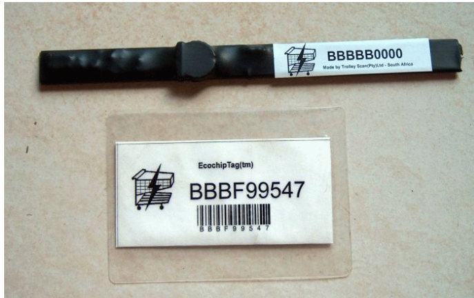
Stick tag and credit card sized transponders
