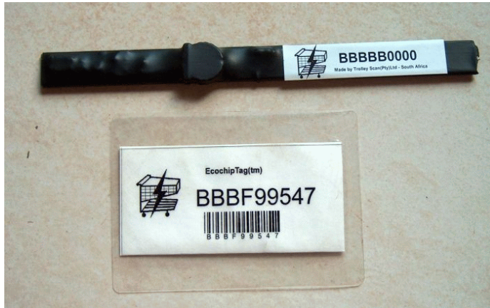
Stick tag and credit card sized transponders
